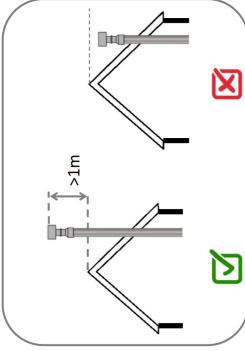
4°.- Installation in masonry chimney, flue up to the exterior.
